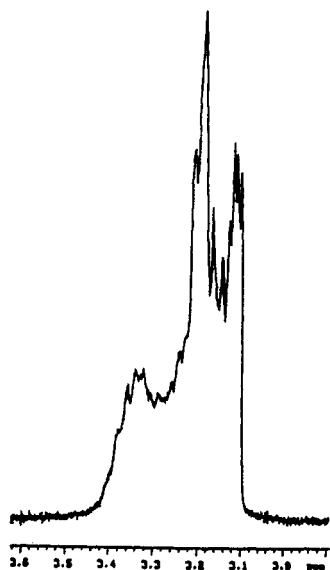
Figure 3. NMR spectra of \text{CH}_2\text{OCH}_3 groups of model polymer E ( M_n = 1800 , M_w/M_n = 1.12 ). (a) ^1\text{H} NMR and (b) ^{13}\text{C} NMR \text{CH}_2\text{O} groups; (c) ^{13}\text{C} NMR \text{OCH}_3 groups.
